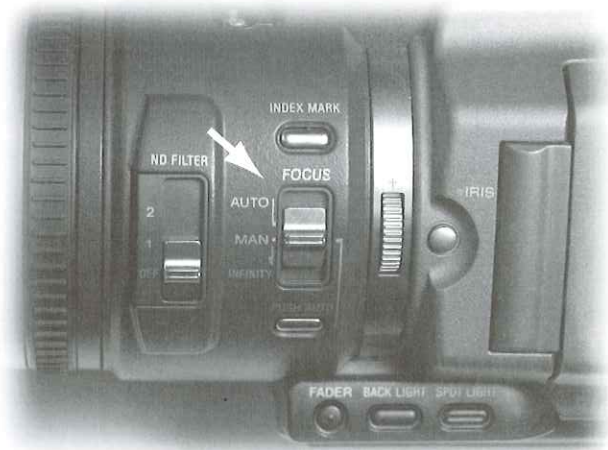
■ Figure 10-25 Most video cameras have a way of switching from automatic to manual focusing, an important feature for maintaining complete control over the way your images are recorded.
