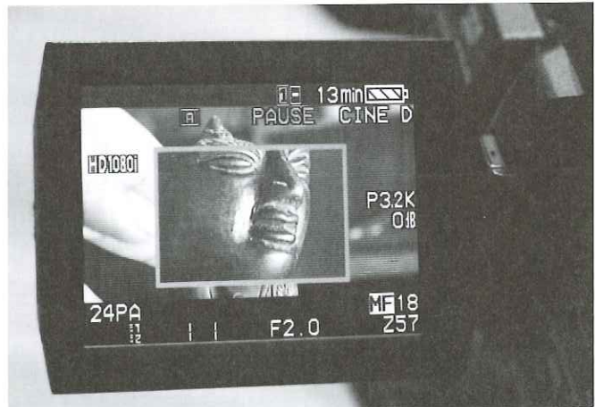
■ Figure 10-12 Camera-to-subject distance is measured from the film plane engraving, found on all film cameras, to the subject (left). To aid with critical focus, some video cameras offer a focus assist function, which magnifies a portion of the scene (right).
