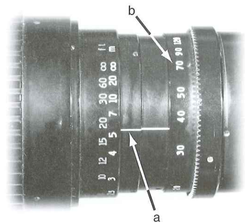
■ Figure 10-9 The focusing ring on a lens has a series of distances engraved in both feet and meters, which are aligned to a witness mark (a) as a reference point. Etched into the zoom ring are the focal length settings in millimeters (b).
