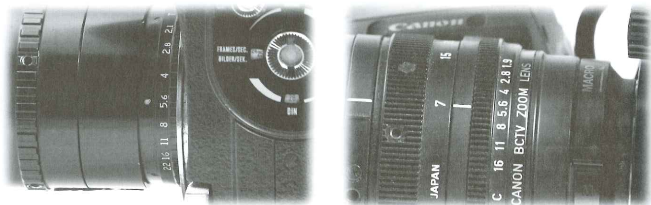
■ Figure 10-17 Both film and high-end video lenses have engraved aperture f-stops for precise control over the incoming light.
