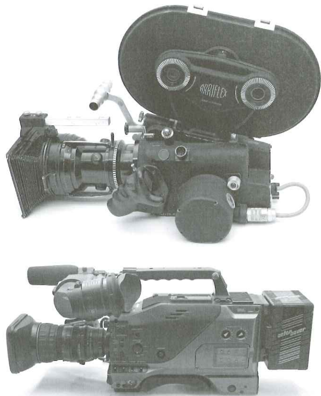
■ Figure 10-7 Zoom lenses have variable focal lengths and provide great flexibility during shooting at the cost of some quality; they are widely available for film cameras ( top ) and standard on video camcorders ( bottom ).
